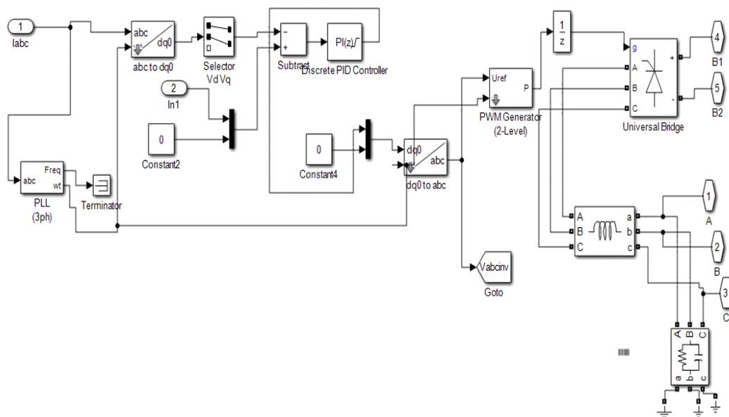
**Figure-3:** Simulation model of proposed PI controller.
