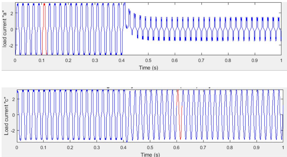
Figure6 Output of proposed topology for unbalanced non-linear loading
