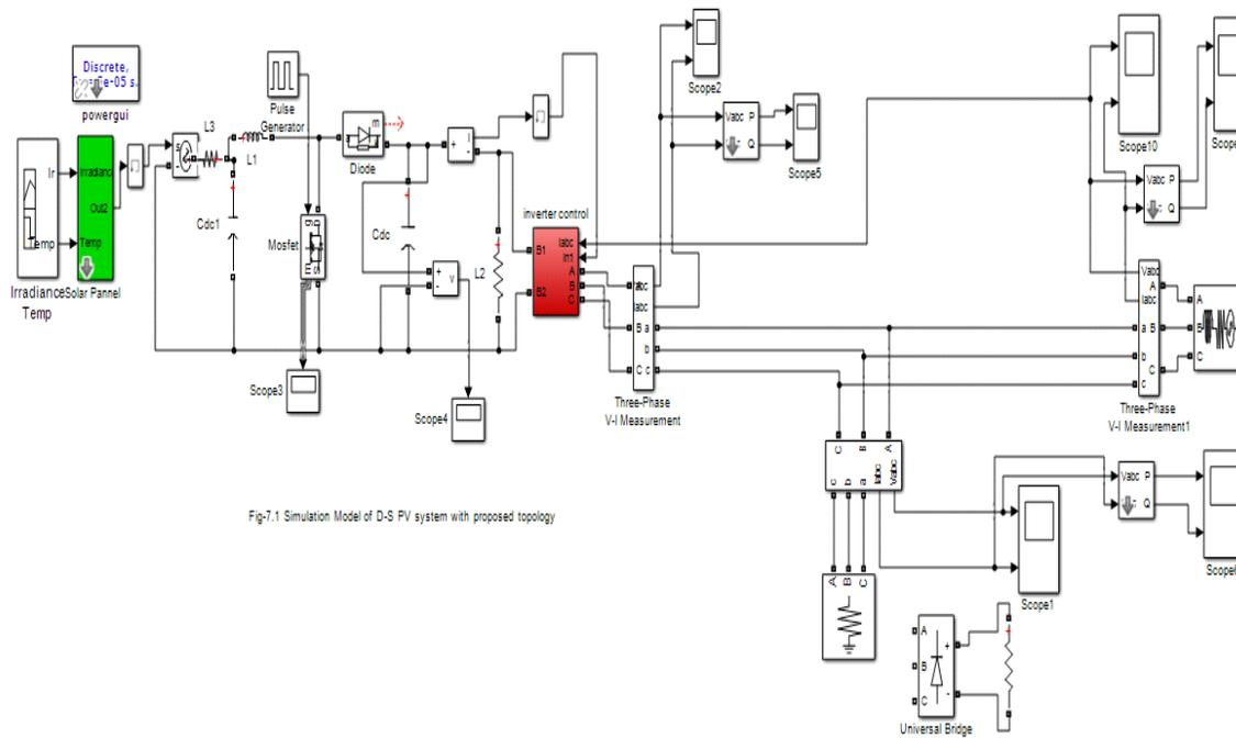
Fig-7.1 Simulation Model of D-S PV system with proposed topology
