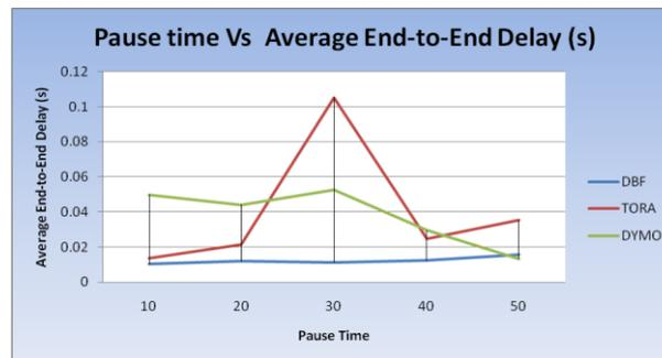
Fig. 2 End to End delay vs Pause Time
