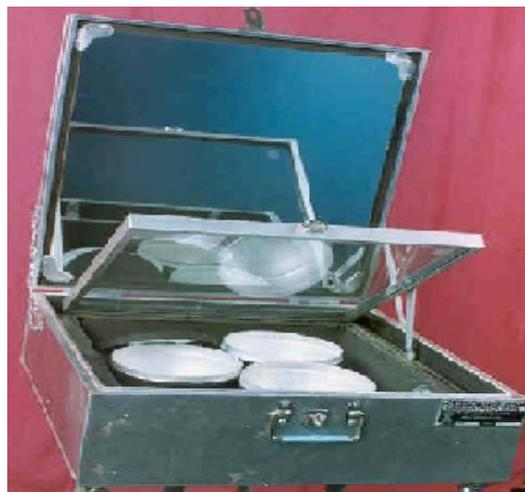
Fig. 2 Box type solar cooker with engine oil as heat storage developed by Nahar [3]
