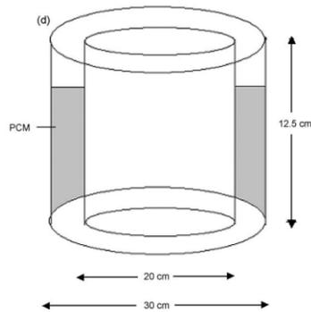
Fig. 6 cylindrical PCM storage unit for a box type solar cooker developed by Buddhi and Sharma [7].
